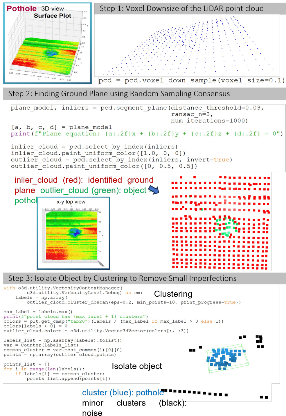
Fig. 8. Ground detected using RANSAC with the pothole identified as an outlier point cluster.
