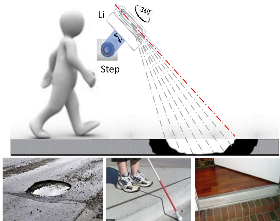
Fig. 1. Conceptual drawing: homemade 3D LiDAR scanner in this project for uneven road surface detection for the visually impaired.
